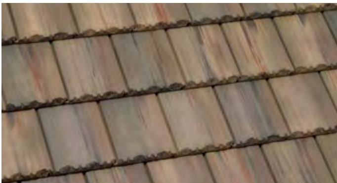
49634 Kings Canyon Blend - Blend of Dark Green, Tan, Red and Black Streaks T24 Ref.13 A.Ref.17 Emi.94 A.Emi.92 SRI12 A.SRI16 CRRC 0918-0044
